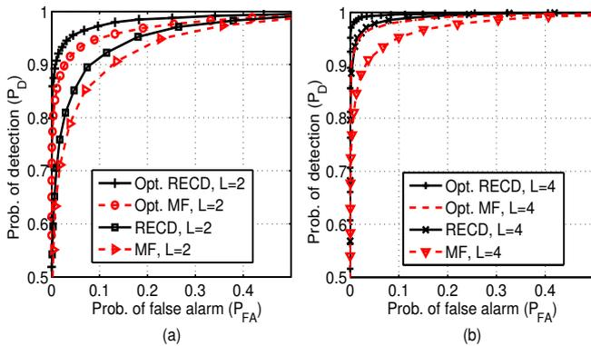
Fig. 3. Comparison of detection performance with optimal beacon signalling versus conventional beacon signaling for the robust estimator-correlator detector (RECD) and matched filter (MF) for  $N_r = 2$ ,  $N_t = 2$  MIMO,  $N = 2$ ,  $\text{SNR} = -5\text{dB}$ ,  $\mathbf{R}_u = \mathcal{D}(1, 0.9)$  (a)  $L = 2$  and (b)  $L = 4$ .
