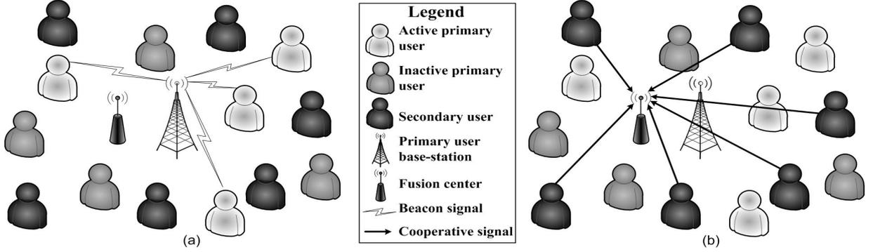
Fig. 1. (a) Cognitive Radio (CR) Network with active and inactive primary users and sensing secondary users, (b) Secondary users cooperate to convey the sensed data to the fusion center for primary user detection.
