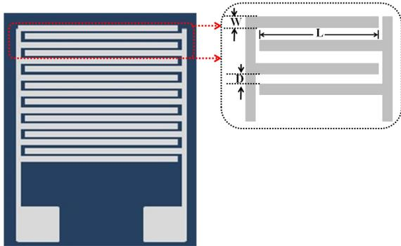
Fig. 2. Micro-Interdigitated electrode array along with its dimensional parameters. From the figure it is clear that for present sensor system  $N=17$ .
