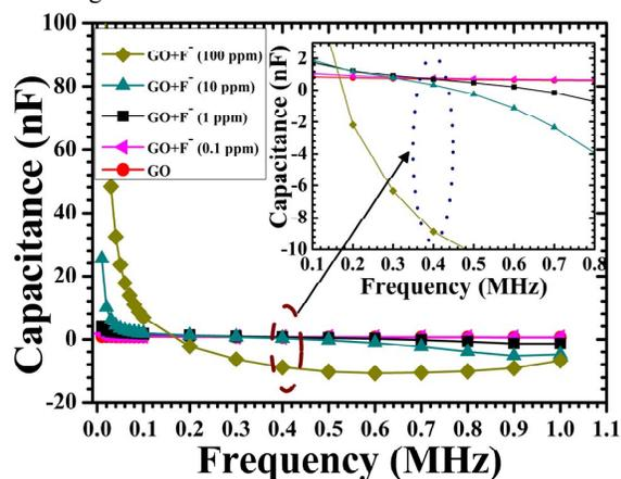
Fig. 8. Capacitance-frequency (C-F) Characteristics for GO-Al- $\mu$ - IDE with GO and GO+ $F^-$  measured up to 1.1 MHz, with fluoride concentration ranging from 0.1-100 ppm. Inset shows the enlarged C-F curves for GO and GO+ $F^-$  with in frequency range (0.1-0.8 MHz)
