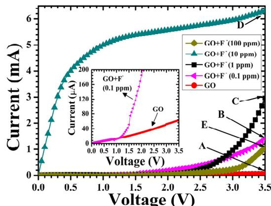
Fig. 7. Current -Voltage (I-V) Characteristics for GO-Al-μ-IDE with GO and GO+F measured up to 3.5 V, with fluoride concentration ranging from 0.1-100 ppm. Satellite shows the enlarged I-V curves for GO and GO+F (0.1 ppm)
