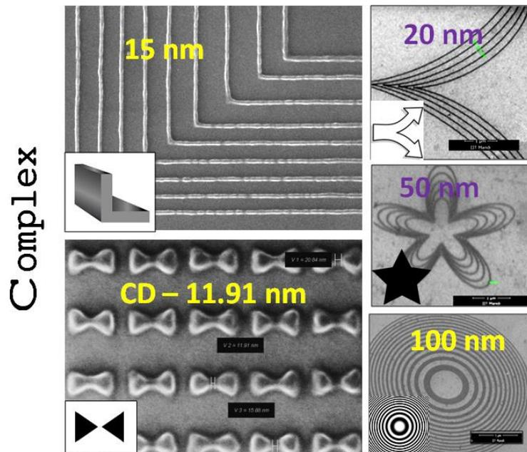
Figure 7 Complex patterning on MAPDST-Ag for different NEMS/MEMS applications; L shape, arrow, star, ring, and nano-boat; the inset shows images of design file patterned over MAPDST-Ag.
