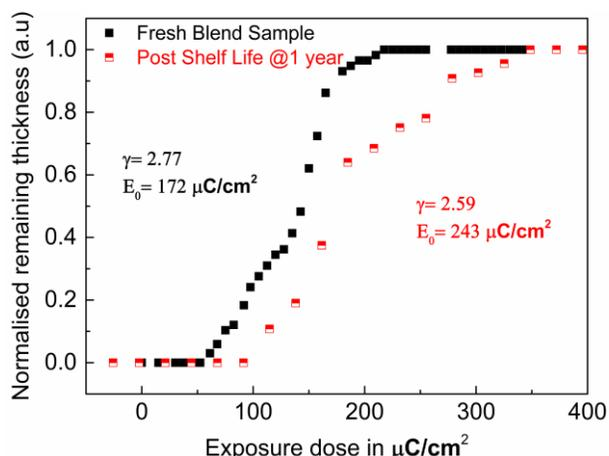
Figure 8 Normalised remaining thickness vs. sensitivity curve for MAPDST-Ag fresh sample and post shelf life (1 year)
