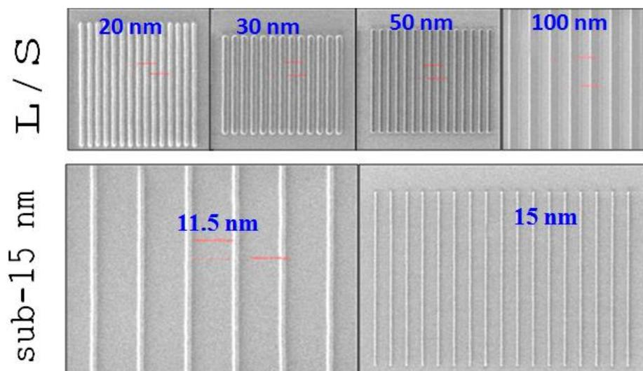
Figure 6 High-resolution patterning with  $\text{He}^+$ IBL; Line space pattern of 20 nm, 300 nm, 50 nm, 100 nm on MAPDST-Ag. Isolated lines of 11.5 nm and 15 nm with ultra-low LER
