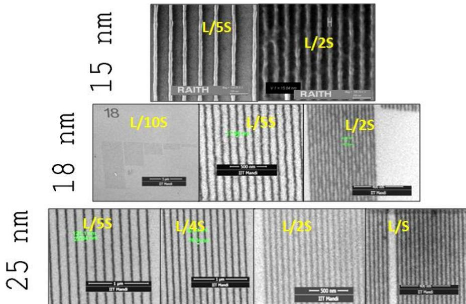
Figure 5 E-beam pattern exposed with dose  $200 \mu\text{C}/\text{cm}^2$  with different feature size and spacing; 15 nm with L/5S and L/2S; 18 nm L/10S, L/5S and L/2S; 25 nm L/5S, L/4S, L/2S, L/S patterns
