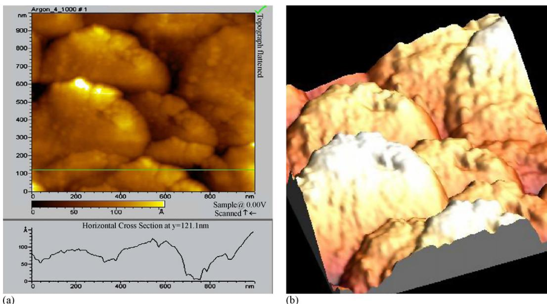
Fig. 5. 2D and 3D AFM images of argon PIII treated silicon surface.
