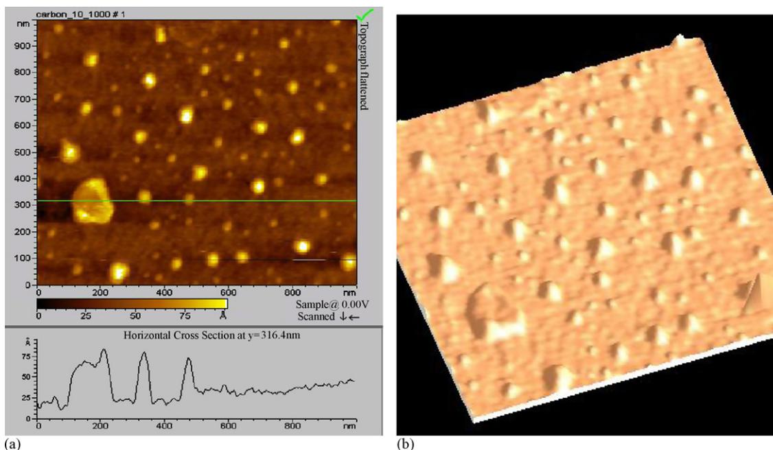
Fig. 2. 2D (a) and 3D (b) AFM images of carbon PIII treated silicon surface.
