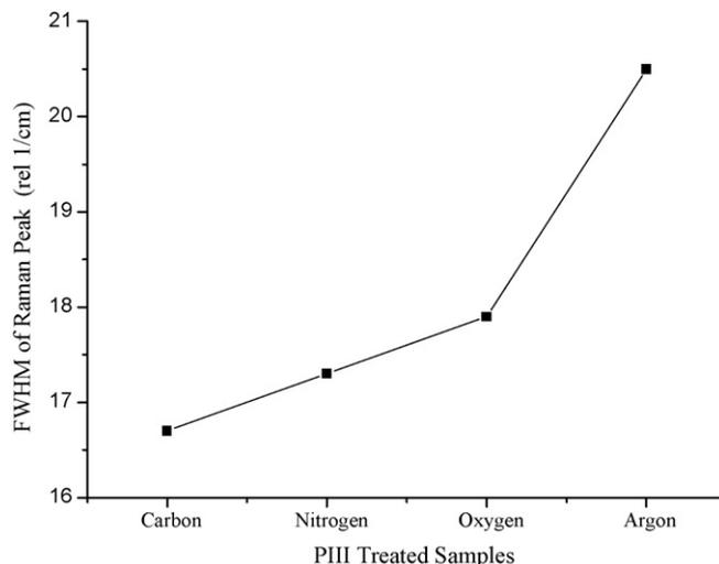
Fig. 9. FWHM of the Raman spectra of the PIII treated samples.
