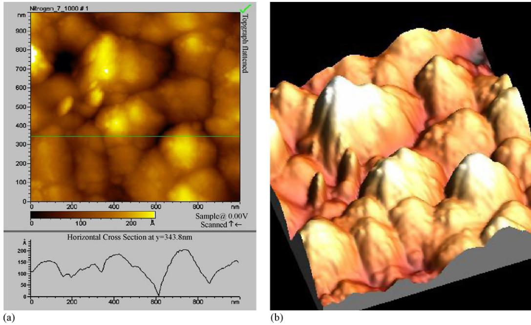
Fig. 3. 2D (a) and 3D (b) AFM images of nitrogen PIII treated silicon surface.
