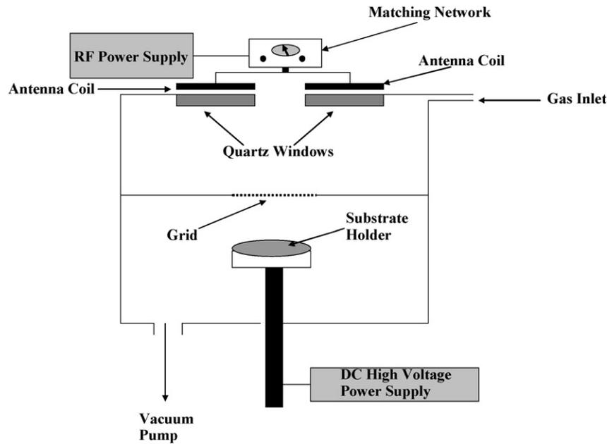
Fig. 1. Schematic representation of plasma immersion ion implantation system.
