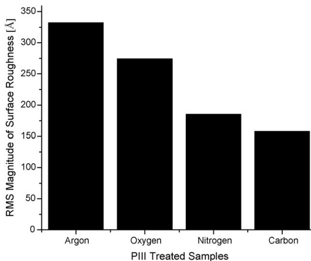
Fig. 6. Surface roughness [RMS (Å)] of PIII treated silicon wafers.
