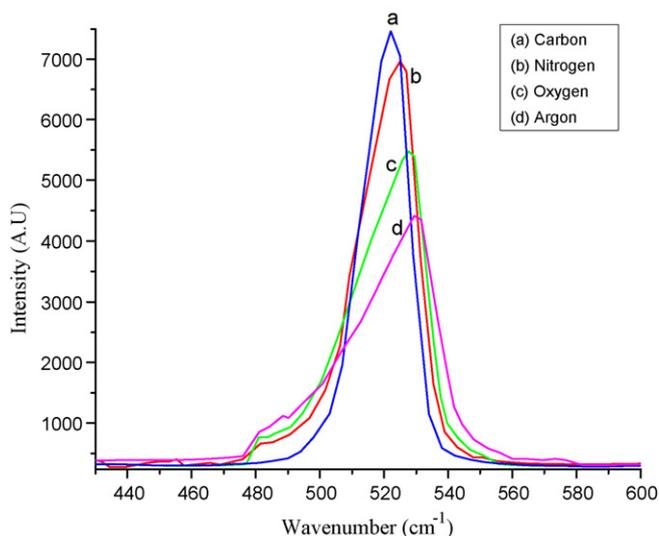
Fig. 7. Raman spectra of the carbon, nitrogen, oxygen and argon PIII treated silicon substrates.
