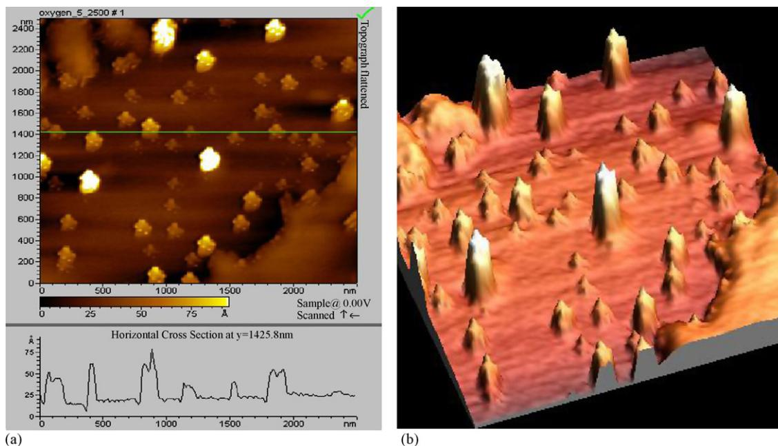
Fig. 4. 2D (a) and 3D (b) AFM images of oxygen PIII treated silicon surface.
