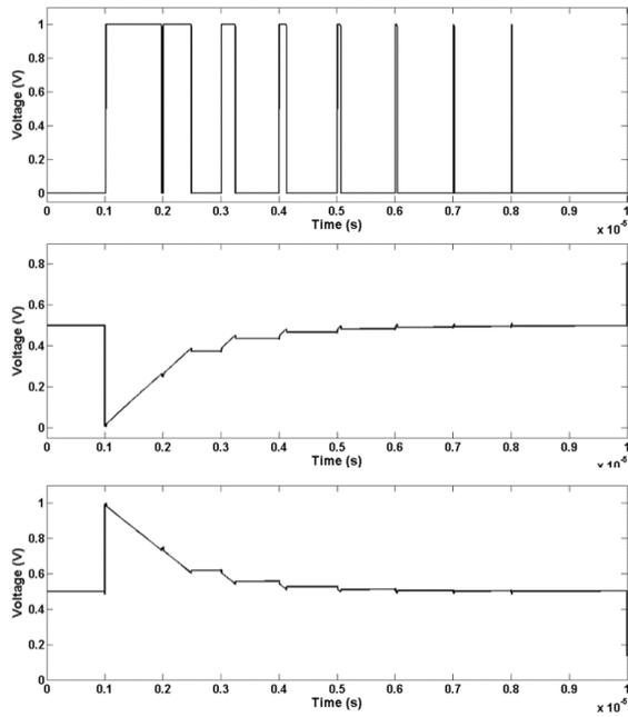
Figure 8. ADC Control Signal,  $V_{CAP}$  when  $V_{IN} = 1$  and  $V_{IN} = 0$ .
