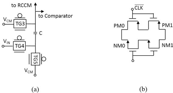
Figure 2. (a) Input Sampling Implementation, (b) Stacked Transmission Gate.
