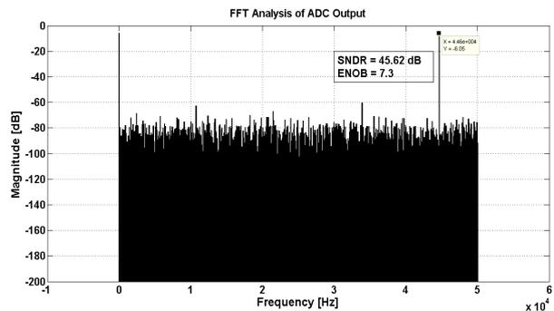
Figure 7. FFT Spectrum (1024 points) at 100 ks/s for input frequency of 44.63 kHz and supply voltage of 1V.
