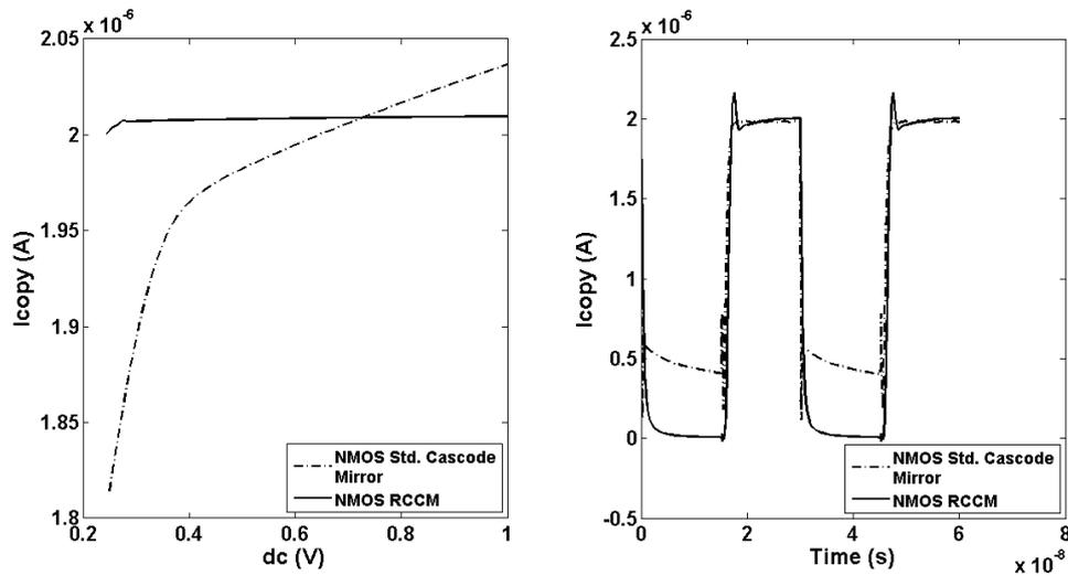
Figure 5. DC and transient analysis of standard NMOS Cascode mirror and NMOS regulated clocked current mirror..
