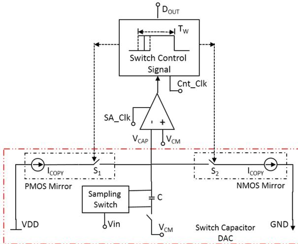
Figure 4. Switch-capacitor DAC ADC architecture.
