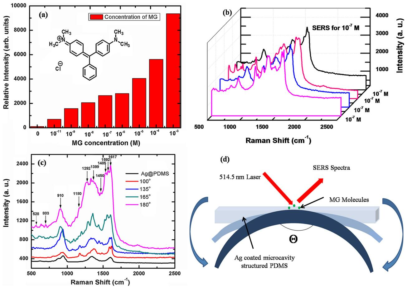
**Fig. 6.** (a) SERS intensity of Ag/PDMS system for 1617 cm<sup>-1</sup> peak with variation in MG concentration, and (b) SERS spectra of 10<sup>-7</sup> M, MG measured at four randomly selected locations on Ag/PDMS substrate, (c) The SERS spectra of the 10<sup>-7</sup> M, MG concentration with different bending angle (strain) (d) schematic representation of the SERS substrate bending and the measurement of the SERS spectra.
