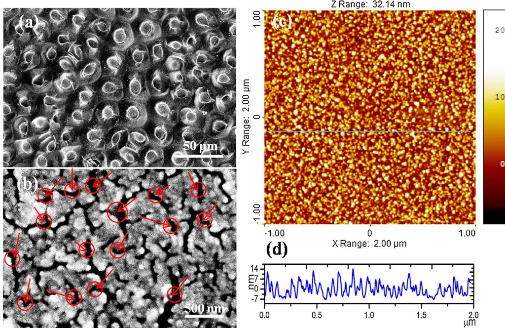
**Fig. 4.** (a) FESEM image of Ag-coated structured Ag/PDMS specimen (b) a higher magnification FESEM image in (a), (c) AFM image ( $2 \mu\text{m} \times 2 \mu\text{m}$ ) of Ag film deposited on non-structured smooth PDMS surface and (d) is the line profile measurement on the AFM image.
