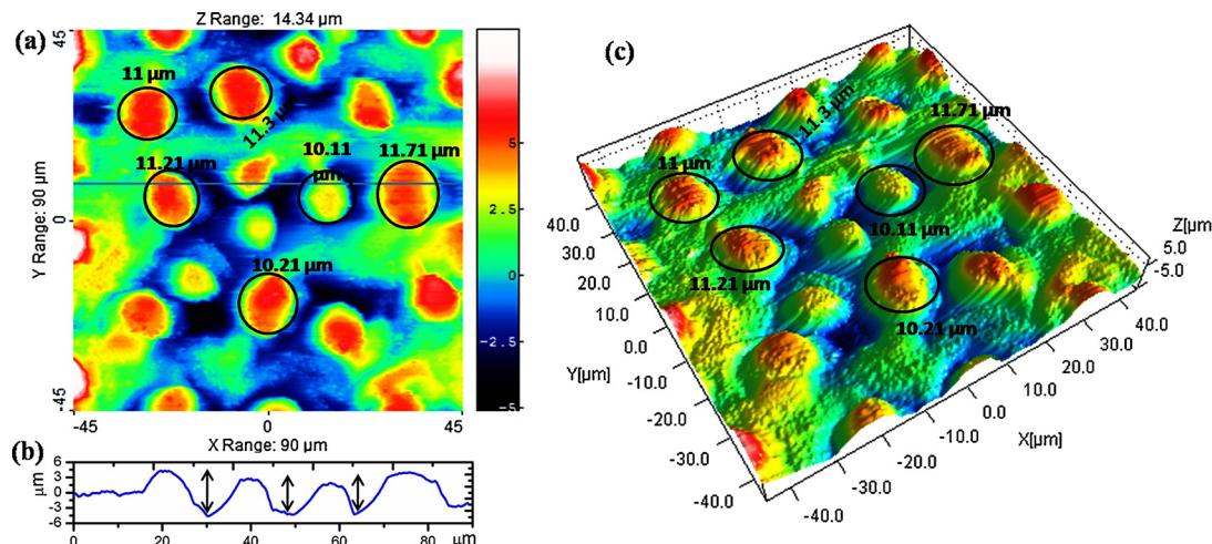
**Fig. 2.** (a) AFM 2D topography ( $90 \mu\text{m} \times 90 \mu\text{m}$ ) image of Taro leaf surface, (b) the line profile measurement on the AFM image and (c) 3D AFM image ( $90 \mu\text{m} \times 90 \mu\text{m}$ ).
