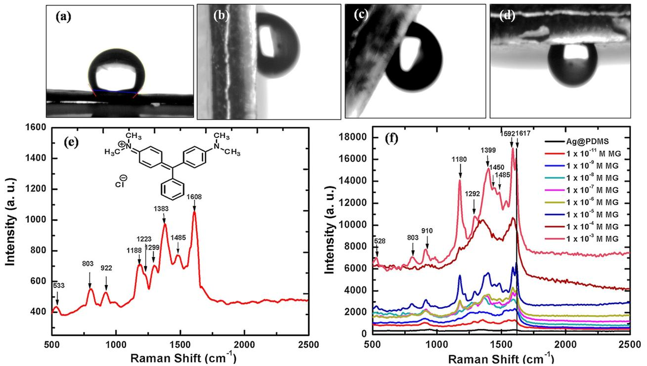
**Fig. 5.** Contact angle and adhesion measurement at different tilted angle (a)  $0^\circ$ , (b)  $90^\circ$ , (c)  $65^\circ$ , (d)  $180^\circ$  on the surface of microcavity structure Ag/PDMS substrate. (e) Raman spectra of bulk MG on Si substrate as probe molecule with concentration of 27 mM and (f) SERS spectra of MG on Ag/PDMS substrate for various concentration of MG.
