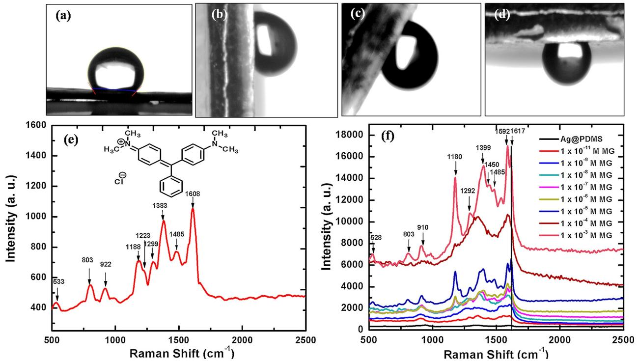
**Fig. 5.** Contact angle and adhesion measurement at different tilted angle (a)  $0^\circ$ , (b)  $90^\circ$ , (c)  $65^\circ$ , (d)  $180^\circ$  on the surface of microcavity structure Ag/PDMS substrate, (e) Raman spectra of bulk MG on Si substrate with concentration of 27 mM and (f) SERS spectra of MG on Ag/PDMS substrate for various concentration of MG.
