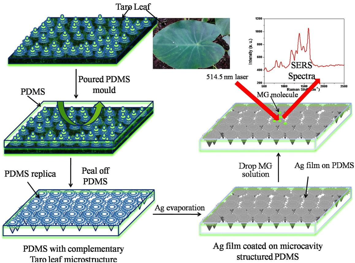
**Fig. 1.** Schematic for the fabrication of Ag decorated micro-cavity array PDMS SERS substrate using Taro leaf as a template.
