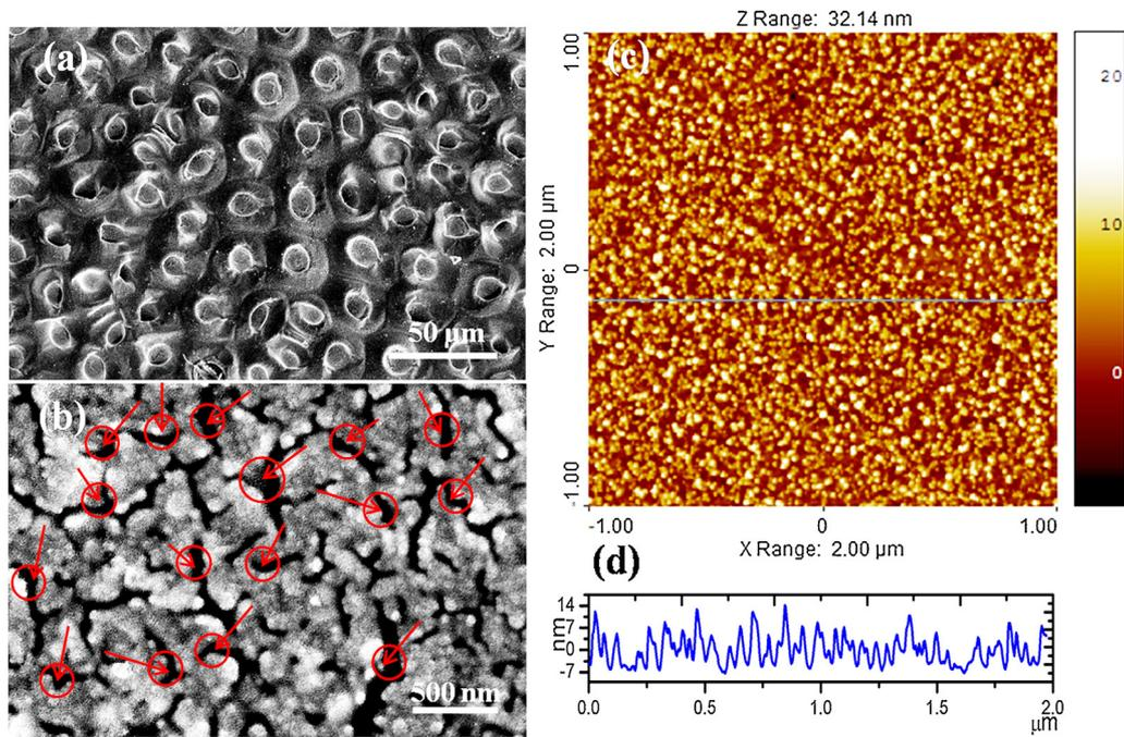
**Fig. 4.** (a) FESEM image of Ag-coated structured Ag/PDMS specimen (b) a higher magnification FESEM image in (a), (c) AFM image ( $2\ \mu\text{m} \times 2\ \mu\text{m}$ ) of Ag film deposited on non-structured smooth PDMS surface and (d) is the line profile measurement on the AFM image.
