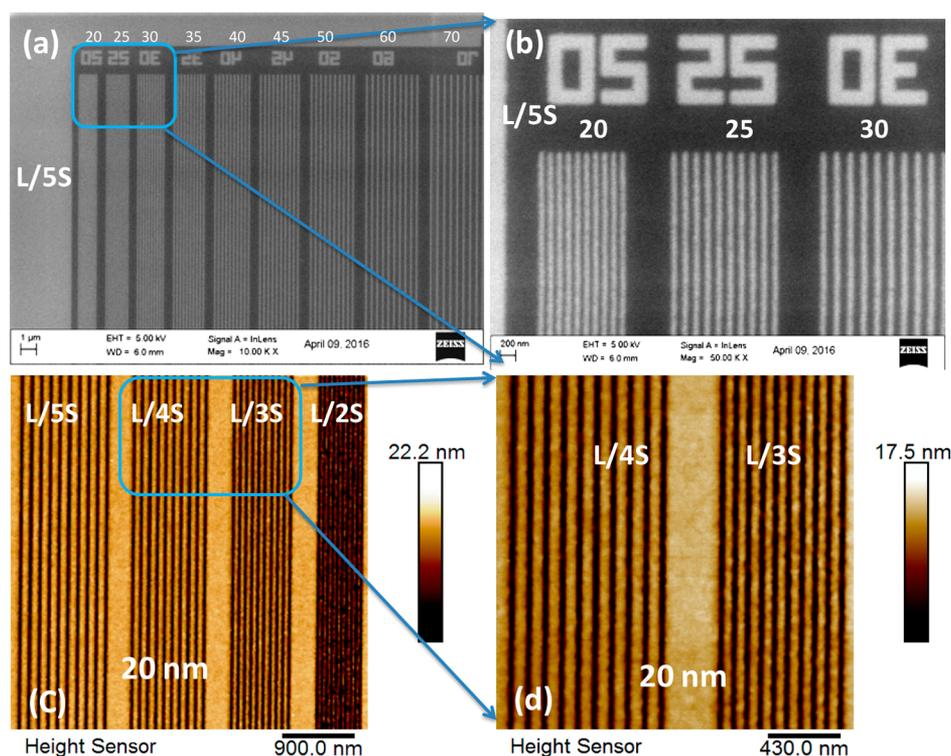
**Figure 2.** (a) FE-SEM image of isolated patterns of 20, 25, 30, 35, 40, 45, 50, 60, and 70 nm with L/5S (line/space) gap; (b) high-magnification image of 20, 25, and 30 nm isolated lines with L/5S; (c) AFM image of 20 nm line patterns with L/2S to L/5S; and (d) high-resolution AFM image of 20 nm line patterns with L/4S and L/3S, CD on the mask.
