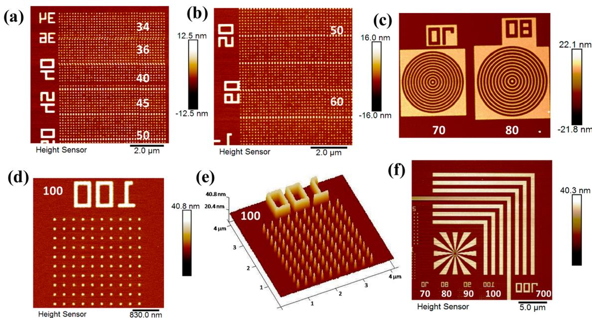
**Figure 3.** HR-AFM complex features of EUV exposed PAS polymer. (a) Highly dense arrays of 34, 36, 40, and 45 nm dots; (b) 50 and 60 nm dots; (c) circular patterns of PAS with 70 and 80 nm features; (d) 100 nm dots; (e) 3D view of 100 nm dots; (f) an image showing star-elbow features.
