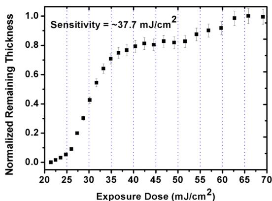
Figure 4. NRT vs EUV dose characteristics of the PAS resist.
