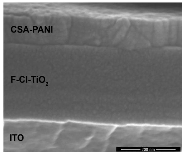
**Fig. 6.** Cross-sectional FE-SEM image of the F-Cl-TiO<sub>2</sub>/CSA-PANI, n-p heterostructure.
