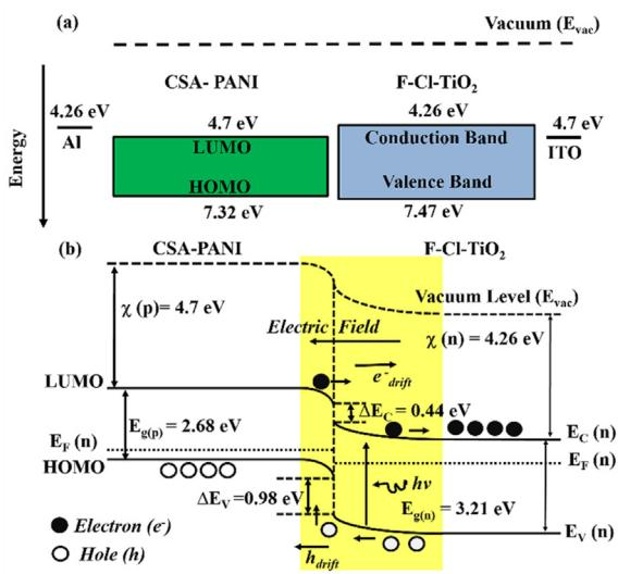
**Fig. 10.** Schematic energy levels of the F-Cl-TiO<sub>2</sub>/CSA-PANI, n-p heterostructure. The energy band diagrams of F-Cl-TiO<sub>2</sub>/CSA-PANI, n-p heterostructure under UV illumination under reverse bias condition.
