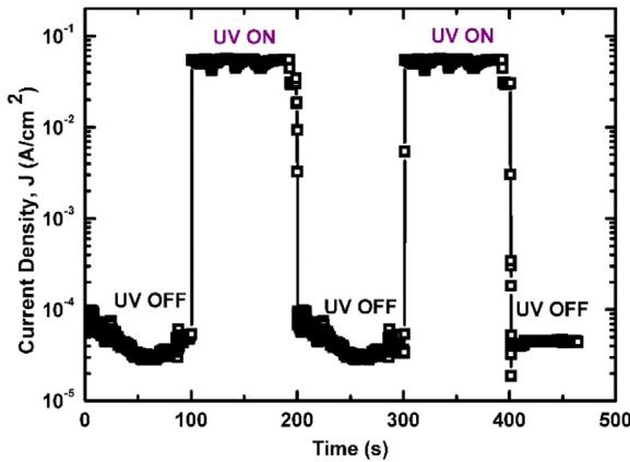
**Fig. 5.** Current density-Time (J-T) Characteristics of Al/CSA-PANI/F-Cl-TiO<sub>2</sub>/ITO, structure at  $-1$  V bias, where the UV light is illuminated after alternate 100 s.
