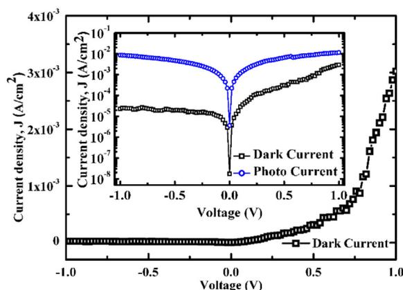
Fig. 3. Current density-Voltage (J-V) Characteristics of Al/CSA-PANI/F-Cl-TiO<sub>2</sub>/ITO, structure. The inset shows the semi-log plot of dark and photo (365 nm illumination) J-V characteristics of Al/CSA-PANI/F-Cl-TiO<sub>2</sub>/ITO, structure.
