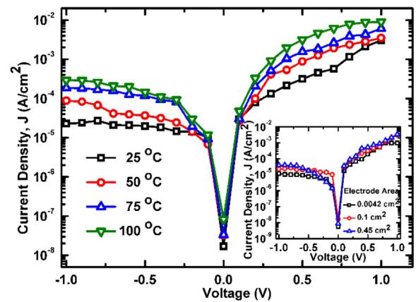
**Fig. 4.** Current density-Voltage (J-V) Characteristics of Al/CSA-PANI/F-Cl-TiO<sub>2</sub>/ITO, structure with variation in temperature of 25, 50, 75 and 100 °C. The inset shows the J-V plots of Al/CSA-PANI/F-Cl-TiO<sub>2</sub>/ITO, structure with variation in Al electrode area.
