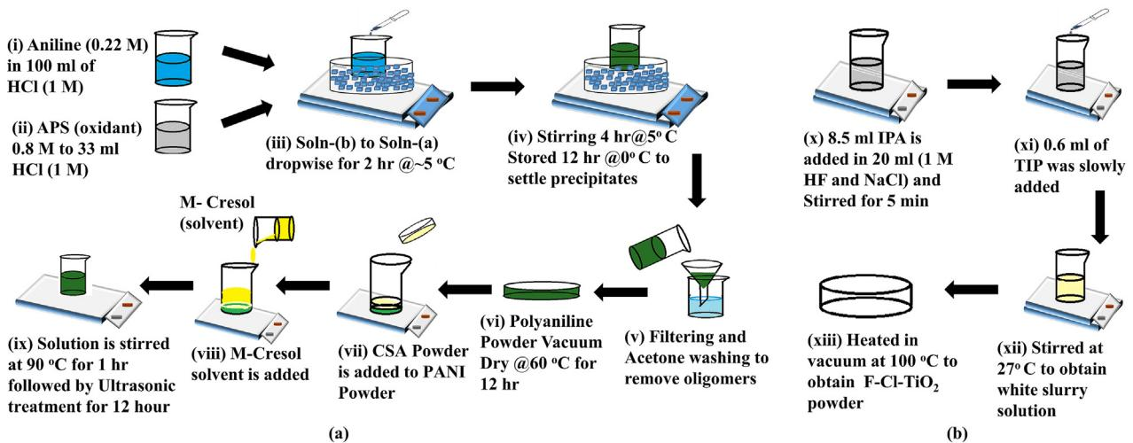
**Fig. 1.** Synthesis of CSA-PANI using Chemical Oxidation method by polymerization of aniline (i)–(ix), (b) Synthesis of F-Cl-TiO<sub>2</sub> using Sol-Gel Method (x)–(xiii).
