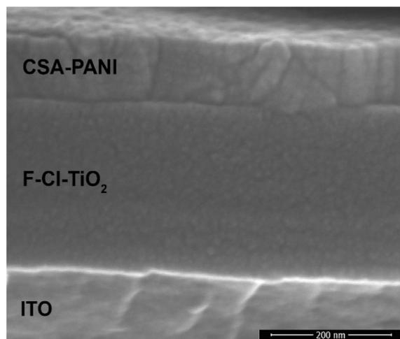
Fig. 6. Cross-sectional FE-SEM image of the F-Cl-TiO<sub>2</sub>/CSA-PANI, n-p heterostructure.
