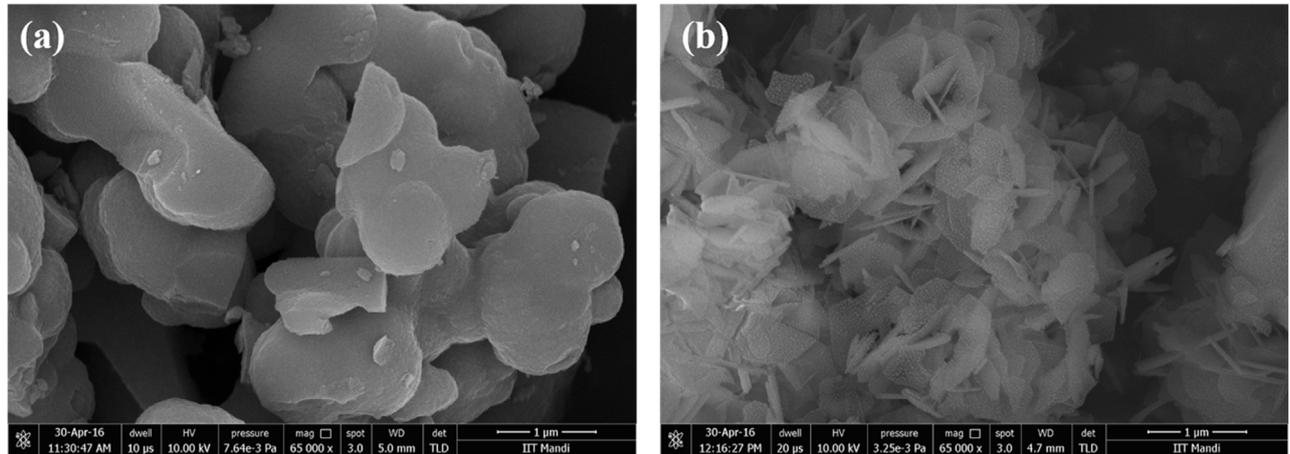
**Fig. 7.** The Surface micrographs of (a) undoped TiO<sub>2</sub> (b) F-Cl doped TiO<sub>2</sub>. The F-Cl doping reduces the surface area as well as porosity in TiO<sub>2</sub> and the flake-like structure confirms the formation of anatase phase in F-Cl-TiO<sub>2</sub>.
