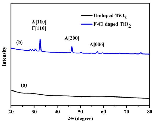
**Fig. 8.** XRD patterns of (a) Undoped TiO<sub>2</sub>, (b) F-Cl doped TiO<sub>2</sub>. The F-Cl doping converts the amorphous phase of undoped TiO<sub>2</sub> to the anatase phase in F-Cl-TiO<sub>2</sub>.
