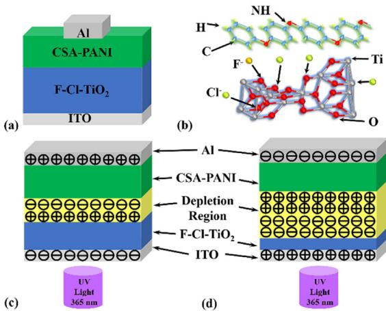
**Fig. 2.** The Al/CSA-PANI/F-Cl-TiO<sub>2</sub>/ITO, organic/inorganic heterostructure device, (a) structure, (b) PANI/TiO<sub>2</sub> crystal structure (C-Blue, H-Yellow, NH-Red in PANI and Ti-Grey, O-Red, F-Yellow, Cl-Green in TiO<sub>2</sub>) (c) under forward bias condition, and (d) under reverse bias condition. (For interpretation of the references to colour in this figure legend, the reader is referred to the web version of this article.)
