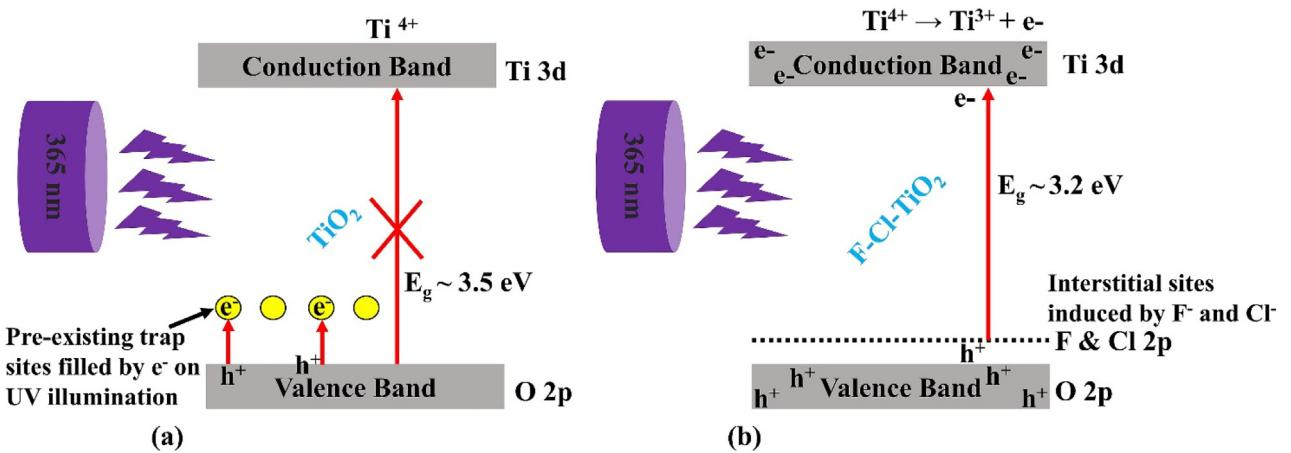
**Fig. 11.** Schematic diagram for (a) undoped TiO<sub>2</sub> and (b) F-Cl doped TiO<sub>2</sub>, showing the proposed mechanism for performance enhancement of photodiode with F and Cl doping in TiO<sub>2</sub>.
