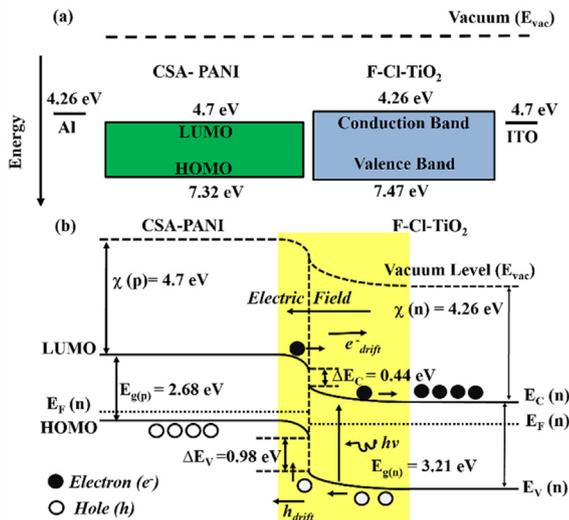
**Fig. 10.** Schematic energy levels of the F-Cl-TiO<sub>2</sub>/CSA-PANI, n-p heterostructure. The energy band diagrams of F-Cl-TiO<sub>2</sub>/CSA-PANI, n-p heterostructure under UV illumination under reverse bias condition.
