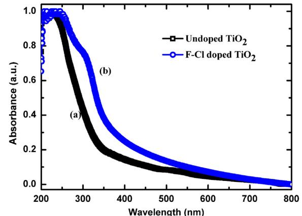
**Fig. 9.** The normalized UV–vis absorption spectra of (a) undoped TiO<sub>2</sub>, (b) F-Cl-TiO<sub>2</sub>. Red (Right) Shift is observed in doped TiO<sub>2</sub>. (For interpretation of the references to colour in this figure legend, the reader is referred to the web version of this article.)
