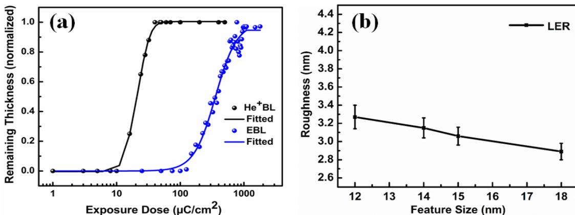
**Figure 3.** (a) Remaining Thickness vs He<sup>+</sup> beam doses characteristics for Ni-DMA MCOC resist, and (b) LER variations with respect to the CD of high dense line patterns.
