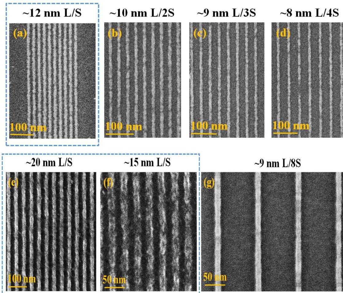
**Figure 1.** FESEM images of exposed Ni-based MCOC resist, using He<sup>+</sup>BL (a) 12 nm L/S (b) 8 nm L/2S patterns and (c) 8 nm L/4S at the dose 40 μC/cm<sup>2</sup>, and using EBL (e)-(f) ~14 nm L/S and (g) ~9 nm L/5S at the dose of ~1400 μC/cm<sup>2</sup>.
