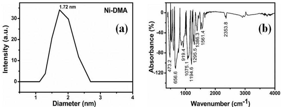
Figure 5. (a) Average cluster size distribution and (b) FTIR of the formulated Ni-DMA MCOC resist.
