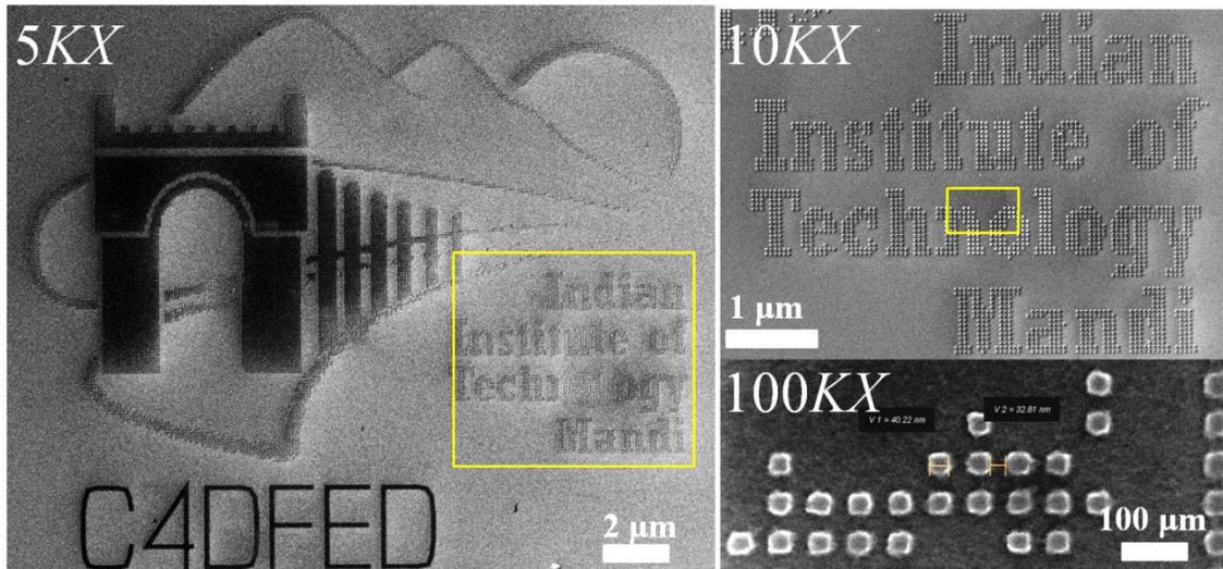
**Figure 2.** FESEM images of EBL exposed complex structure (IIT-Mandi logo) with 40 nm/pixels for logo.bmp and developed ~200 nm alphanumeric sharp-edge structure over Ni-based MCOC resist
