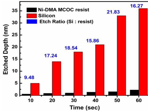
Figure 4. Etched depth with respect to the time for the Ni-DMA MCOC resist and the silicon wafer
