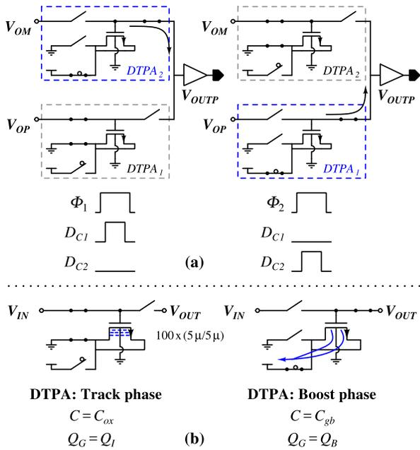
Fig. 4. (a) Working of the interlaced DTPAs in  $\phi_1$  and  $\phi_2$  clock periods and (b) principle of an nMOS DTPA: track and boost phases. In this design, the resulting capacitance of the MOSCAP in the track and boost phases are 12.2 and 3.6 pF, respectively.
