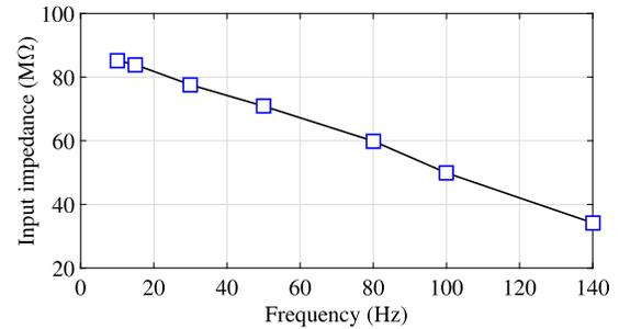
Fig. 20. Input impedance of the amplifier versus input signal frequency.
