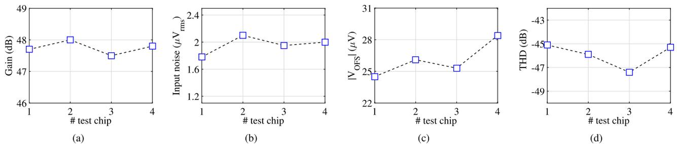
Fig. 21. (a) Gain, (b) input referred noise voltage, (c) input offset voltage, and (d) THD of four chopper-DTPA amplifier chips.
