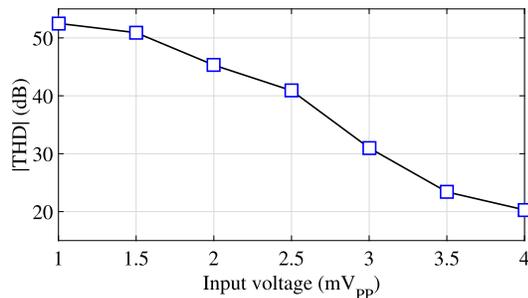
Fig. 19. THD of the amplifier with respect to varying input signal magnitude.
