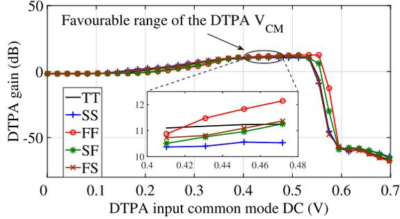
Fig. 11. Simulated DTPA gain with respect to  $V_{CM}$ ; indicating favorable input common mode voltage range across various process corners.
