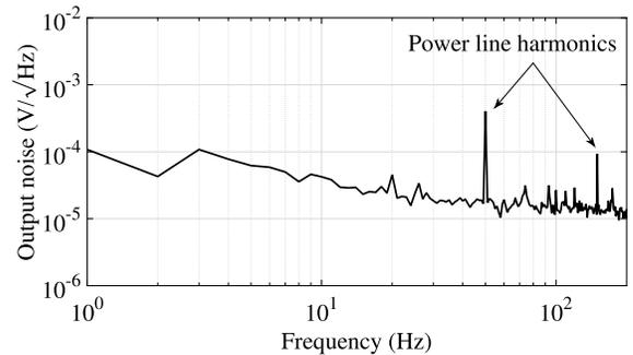
Fig. 17. Measured output noise power spectral density of the amplifier.
