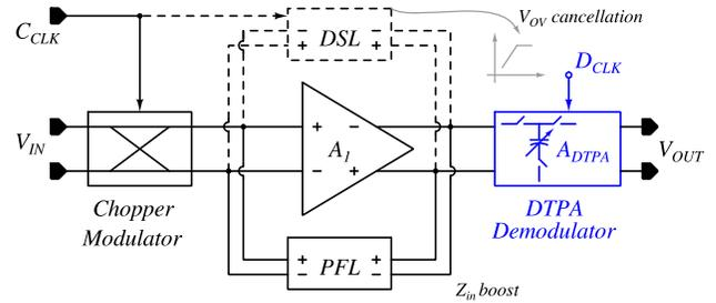
Fig. 2. Architectural block diagram of the proposed chopper stabilized amplifier with DTPA-based signal demodulator.
