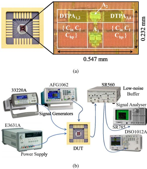
Fig. 15. (a) Microphotograph of the chopper-DTPA amplifier chip and (b) test setup for characterization. (Instrument pictures courtesy: company web pages and the authorized e-commerce web sites).
