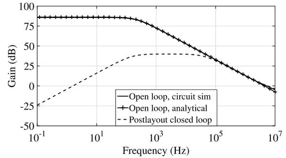
Fig. 6. Analytical and simulated open loop gain of the OTA  $A_1$ , and simulated closed loop response of the capacitively coupled OTA with  $C_{in} = 10$  pF and  $C_f = 100$  fF.
