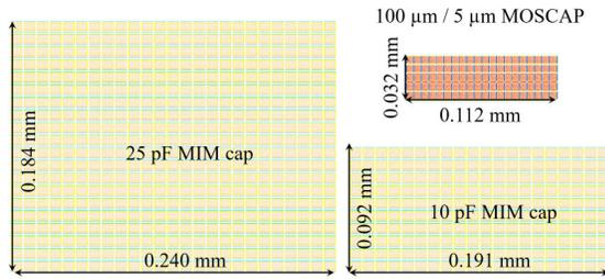
Fig. 22. Layout area of the DTPA MOSCAP in this design, 10 and 25 pF MIM capacitors.
