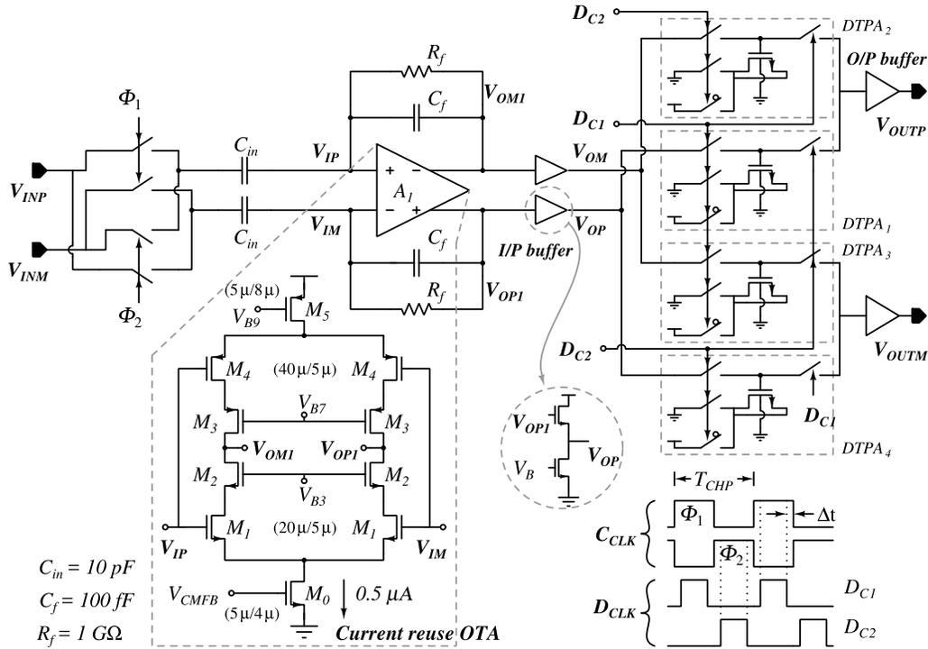
Fig. 3. Circuit implementation of the chopper—DTPA amplifier, the demodulator switching scheme and the clock timing diagram (bias circuitry generating  $V_{B3}$ ,  $V_{B7}$ , and  $V_{B9}$ , and the CMFB for maintaining output common mode of the OTA are not shown here for simplicity).
