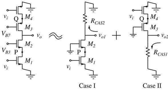
Fig. 5. Equivalent ac half circuit of the current reuse telescopic OTA. Cascode loads are assumed frequency independent for analyzing the frequency response using superposition.
