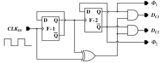
Fig. 12. Implementation of the clock generator circuit to obtain duty cycles of  $C_{CLK}$  ( $\phi_1, \phi_2$ ) and  $D_{CLK}$  ( $D_{C1}, D_{C2}$ ) as 50% and 25%, respectively.
