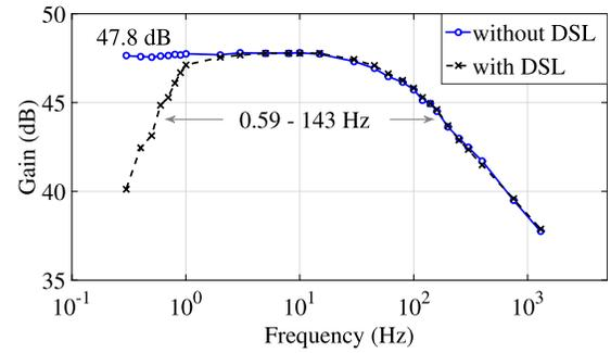
Fig. 16. Transfer characteristics of the amplifier with and without the DSL.
