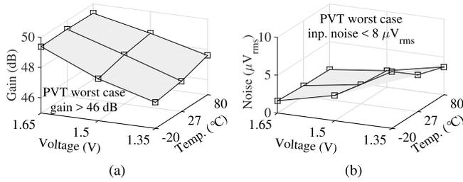
Fig. 14. (a) Gain and (b) input referred noise of the amplifier at SS corner for  $-20^{\circ}\text{C}$  to  $80^{\circ}\text{C}$  temperature with  $V_{\text{DD}}$  varying from 1.35 to 1.65 V.
