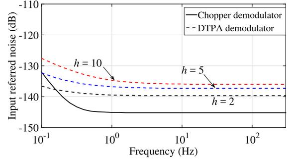
Fig. 13. Input referred noise spectral density of the chopper-DTPA and conventional chopper amplifiers.
