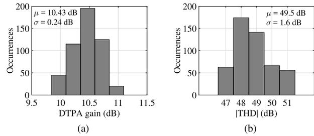
Fig. 9. 500 run Monte Carlo simulation results for (a) DTPA gain and (b) total harmonic distortion of the chopper-DTPA amplifier for  $2 \text{ mV}_{pp}$  signal.
