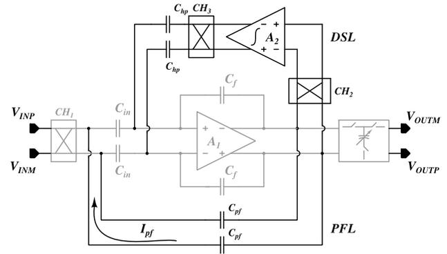
Fig. 7. Implementation of the positive feedback loop and the DSL. An external 1- $\mu$ F capacitor is used in the integrator.
