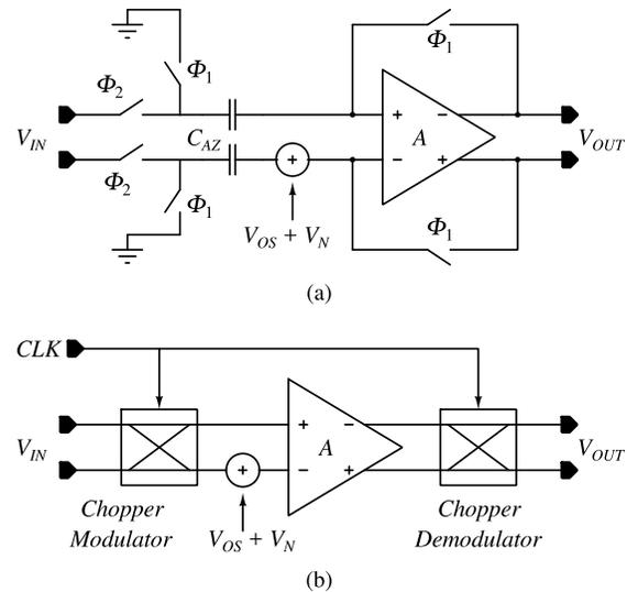
Fig. 1. Simplified block diagrams of the basic (a) auto-zeroed amplifier and (b) chopper amplifier.
