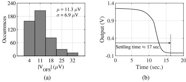
Fig. 8. (a) 500 run Monte Carlo simulation result for offset voltage and (b) settling time of the DSL.
