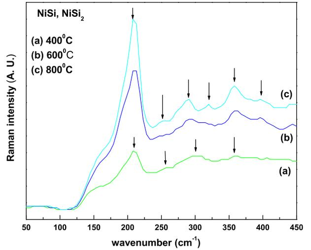
Fig. 3. Raman spectra of NiSi film annealed at different temperatures.
