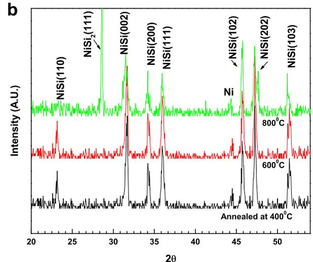
Fig. 2. (a) XRD spectrum of the Si/NiP (50 nm) structure annealed for 30 min at various temperatures. (b) XRD spectrum of the Si/NiP (50 nm) structure annealed 30 min at various temperatures and unreacted nickel metal removed.
