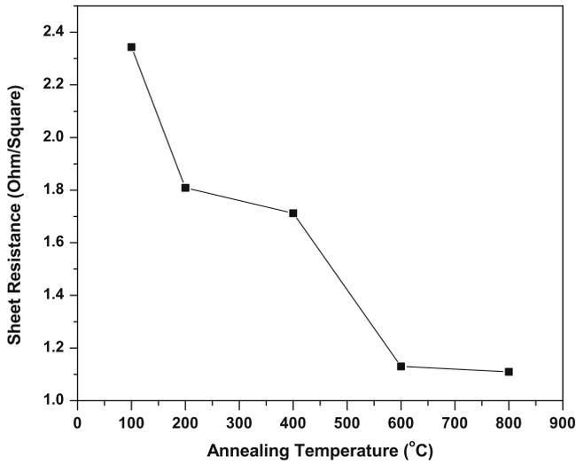
Fig. 1. Variation of sheet resistance with annealing temperature.
