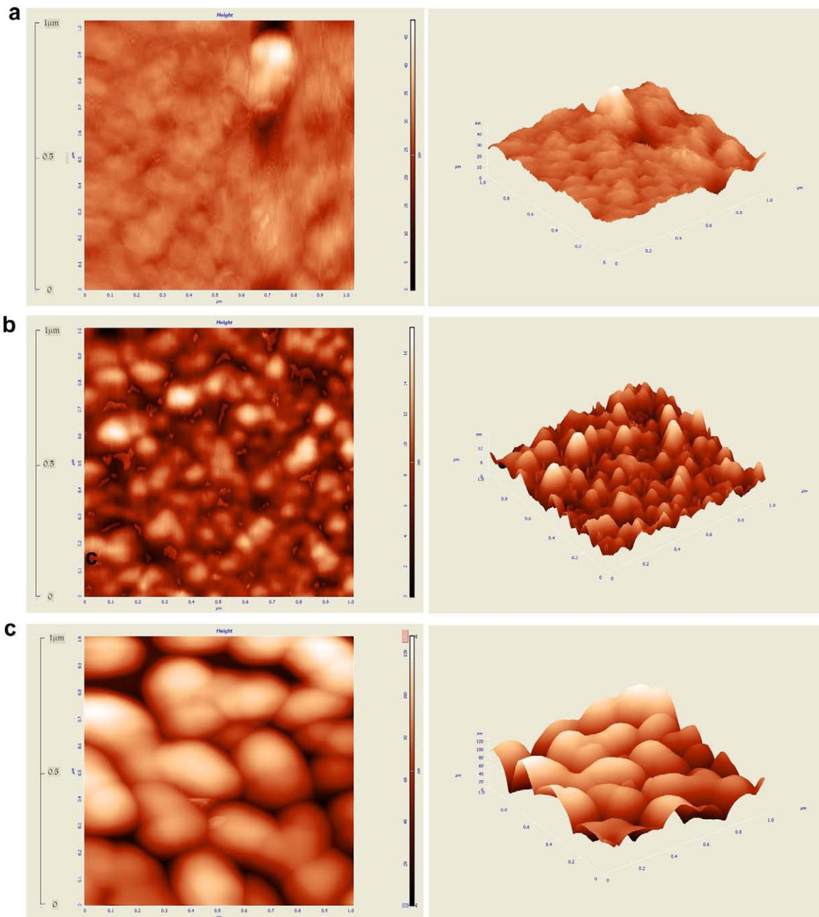
Fig. 4. (a) AFM surface morphology of as deposited Si/NiP sample. (b) AFM surface morphology of  $500^\circ\text{C}$  annealed Si/NiP sample. (c) AFM surface morphology of  $600^\circ\text{C}$  annealed Si/NiP sample.
