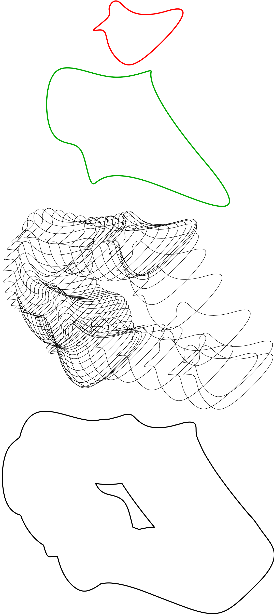
Figure 1: (a) The generator (b) The translation component of motion (c) Generator at a few time instants (d) The boundary of the swept volume.
