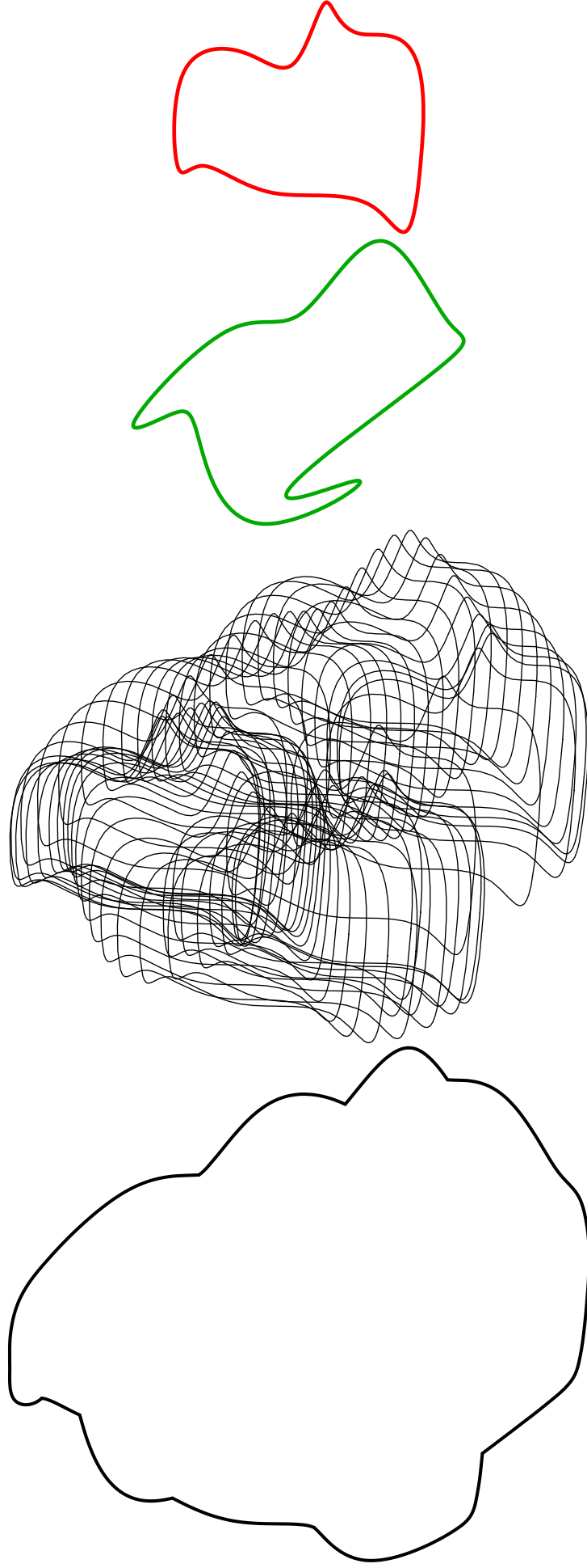
Figure 1: (a) The generator (b) The translation component of motion (c) Generator at a few time instants (d) The boundary of the swept volume.
