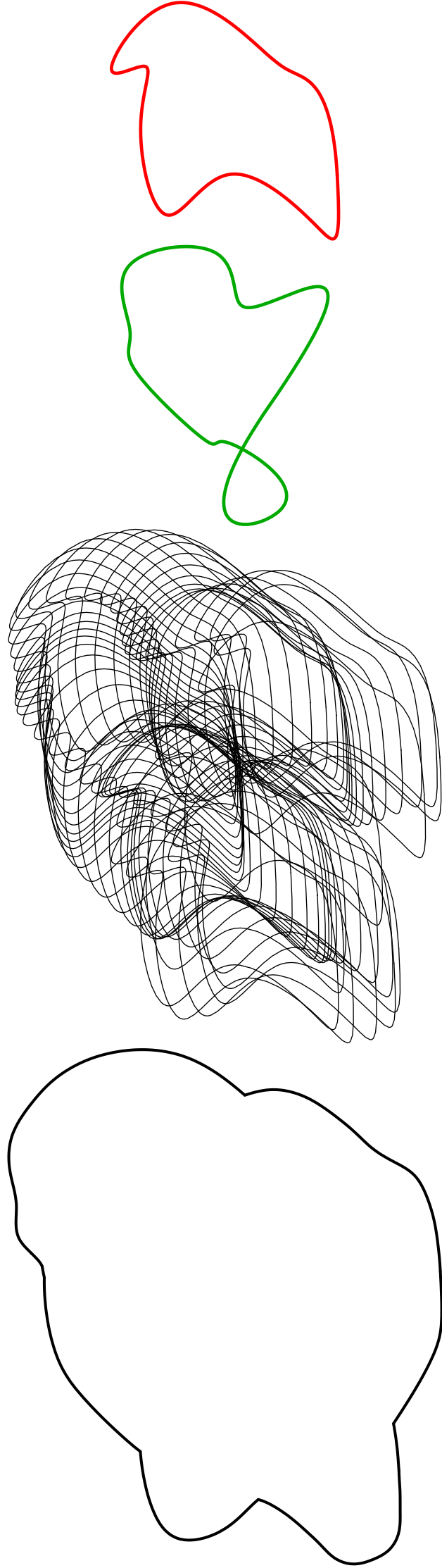
Figure 1: (a) The generator (b) The translation component of motion (c) Generator at a few time instants (d) The boundary of the swept volume.
