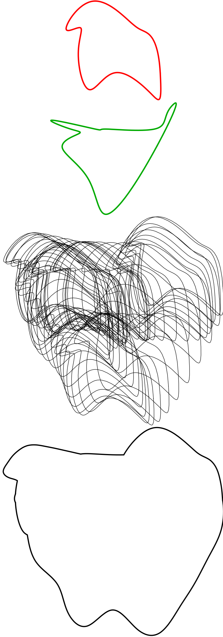
Figure 1: (a) The generator (b) The translation component of motion (c) Generator at a few time instants (d) The boundary of the swept volume.
