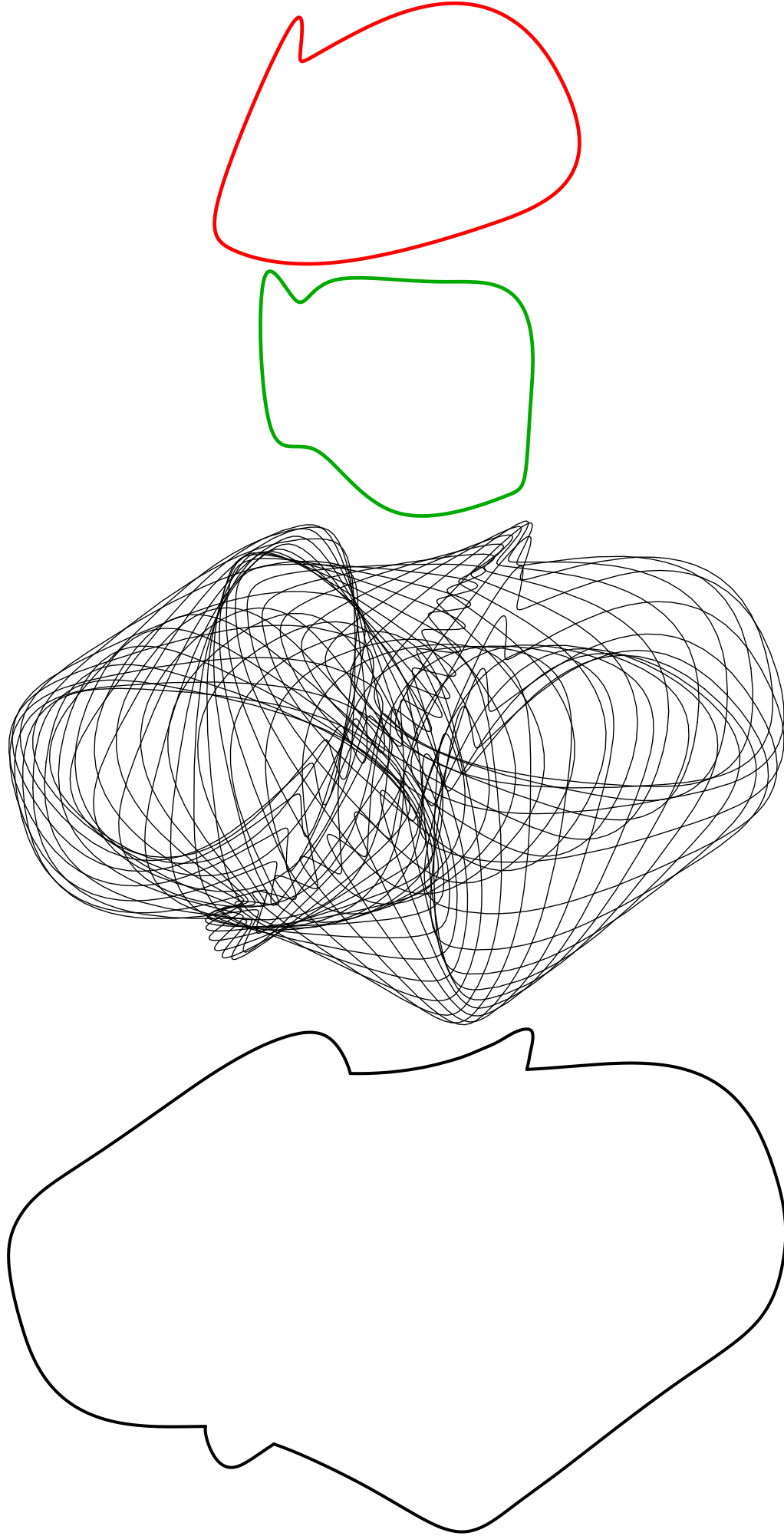
Figure 1: (a) The generator (b) The translation component of motion (c) Generator at a few time instants (d) The boundary of the swept volume.
