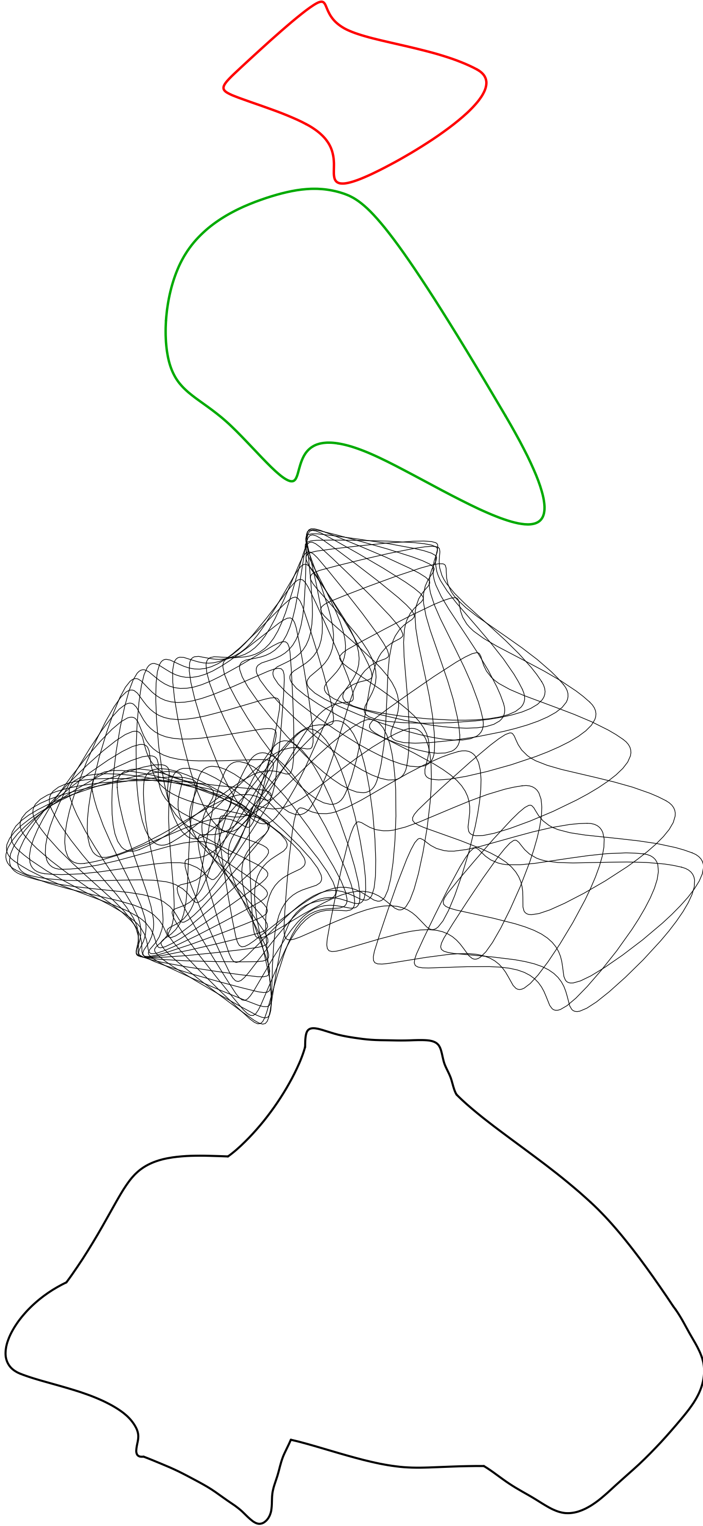
Figure 1: (a) The generator (b) The translation component of motion (c) Generator at a few time instants (d) The boundary of the swept volume.
