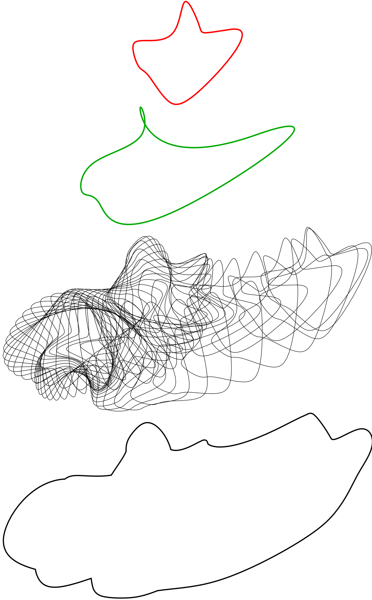
Figure 1: (a) The generator (b) The translation component of motion (c) Generator at a few time instants (d) The boundary of the swept volume.
