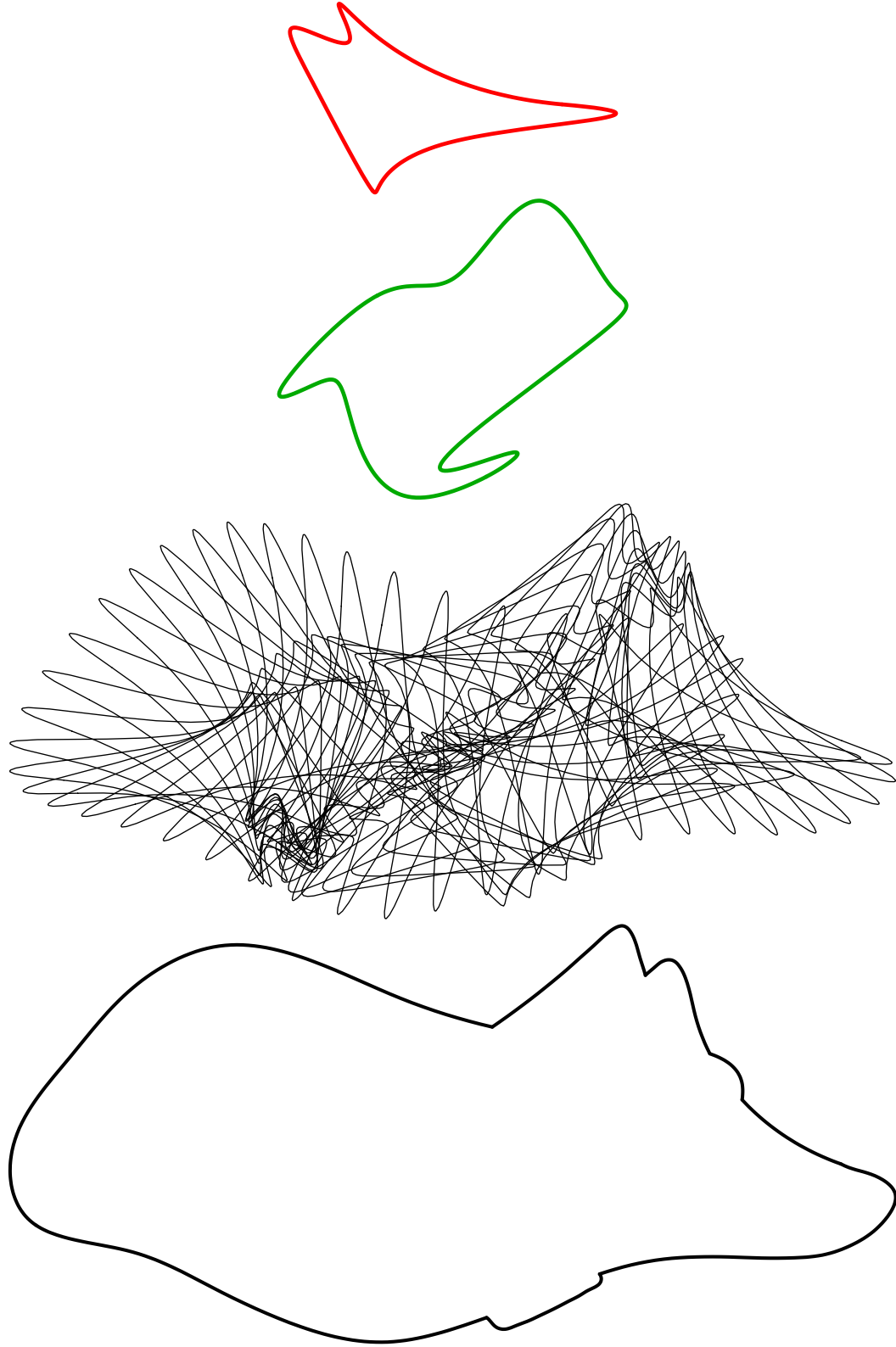
Figure 1: (a) The generator (b) The translation component of motion (c) Generator at a few time instants (d) The boundary of the swept volume.
