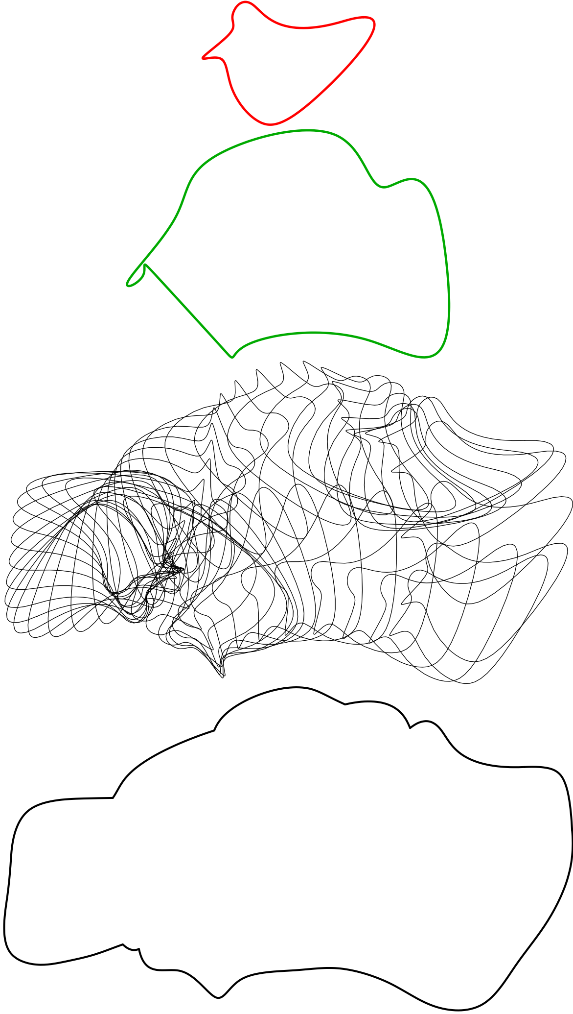
Figure 1: (a) The generator (b) The translation component of motion (c) Generator at a few time instants (d) The boundary of the swept volume.
