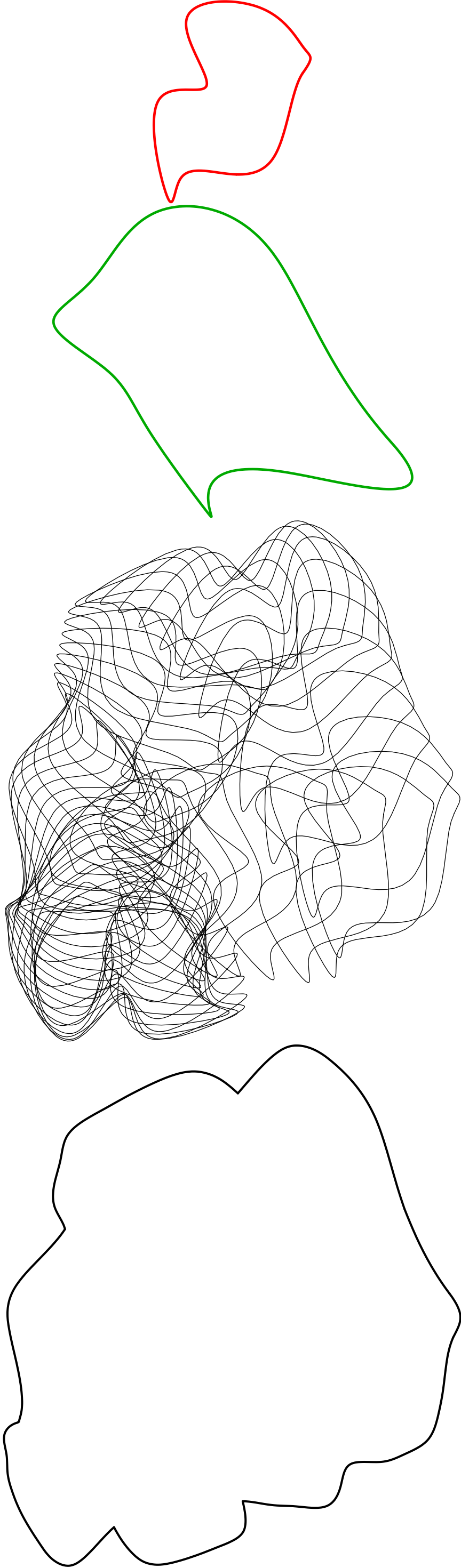
Figure 1: (a) The generator (b) The translation component of motion (c) Generator at a few time instants (d) The boundary of the swept volume.
