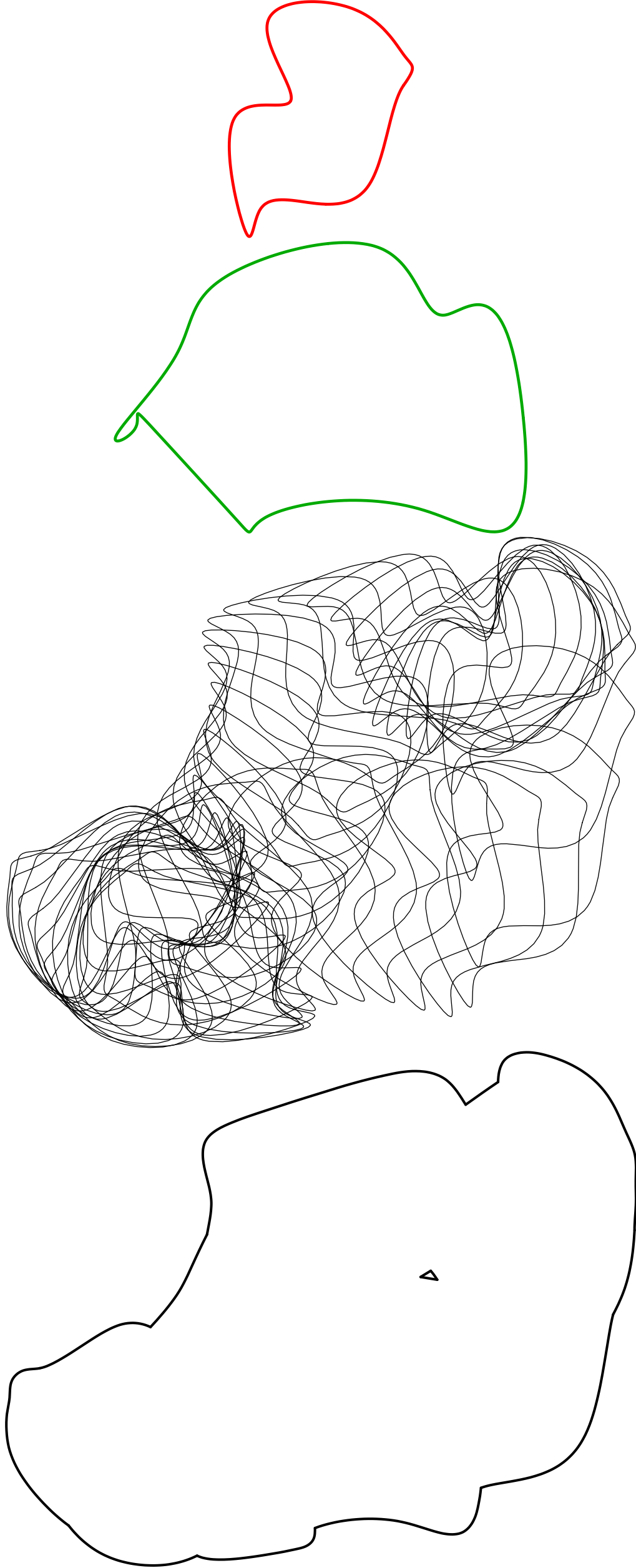
Figure 1: (a) The generator (b) The translation component of motion (c) Generator at a few time instants (d) The boundary of the swept volume.
